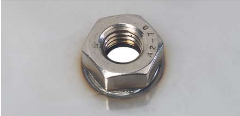
Nut welding onto punched sheet metal
