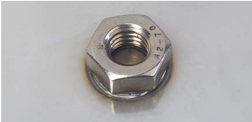
Nut welding onto non-punched sheet metal
