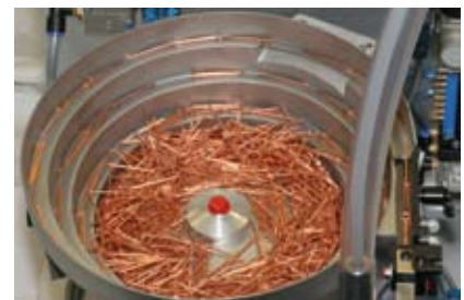
Insulation nails are fed via the bowl feeder and a separator into the feed tube.
