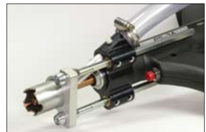
Insulation nails are pneumatically transferred from the feed tube into the nail chuck of the PS-3A welding gun.
